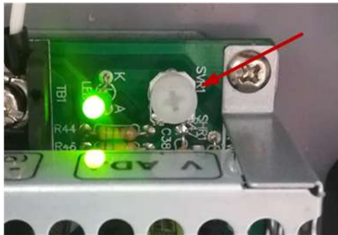
Figure 2 - DC-DC converter adjustment potentiometer
